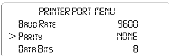
FIG. 4-67 PRINTER PORT MENU/PARITY
