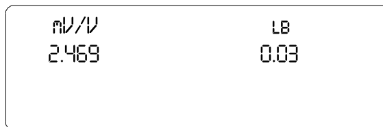
FIG. 7-75 MILLIVOLT/VOLT AND WEIGHT READING
