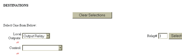
FIG. 6-15 MAPPING SETUP #1 PAGE/SELECTING OUTPUT RELAY #3
